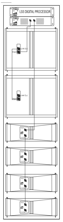
To use an array with ST17 and SB17 is necessary an external digital processor with custom setup provided by LSS. One output channel drive the SB17 and another one drive the ST17. If your amplifier can manage a 2 Ohms Load and has sufficient power, it is possible to connect a maximum of 6 ST17 in parallel per channel (total impedance will be 2 Ohms) or 4 SB17 in parallel per channel
